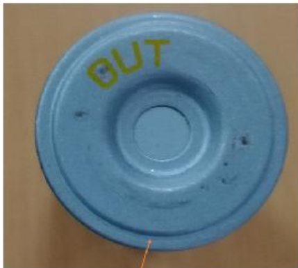
The closed end is the sealed end
