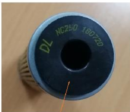
The open end should face the left crankcase.
