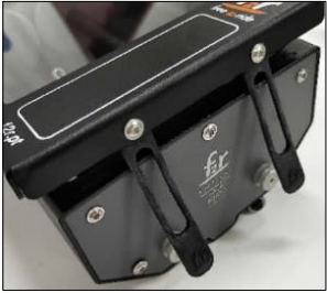
1. Pull down the adhesive strip to open the top cover of the roadbook box
