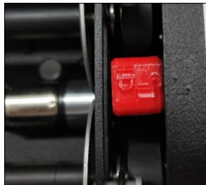
4. Red locking switch button ①Toggle the red button upward to restrict the manual rotation wheel of the roadbook box to turn the pages downward. ②Toggle the red button downward to restrict the manual wheel of the road book box to turn the pages upward.
